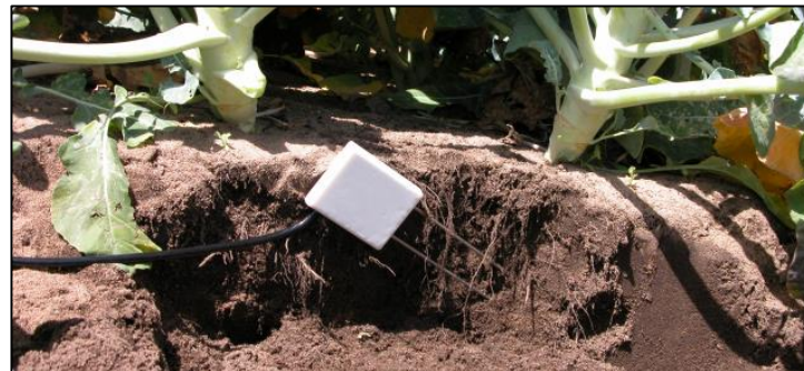
Soil moisture probes
